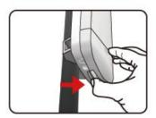
Unlatch the weatherproof sliding door from the rear of the base to open.
